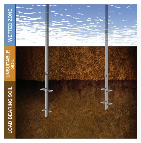
**Example 1**: A helical pile with multiple helices such as a 10"-12"-14" configuration. The largest helix shall determine the additional pile embedment length. In this example the pile must be advanced an additional 3.5 feet of embedment.
