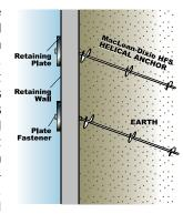
anchors can stabilize walls that have been improperly constructed and can restore walls that have been damaged by poor drainage or expansive soils.
